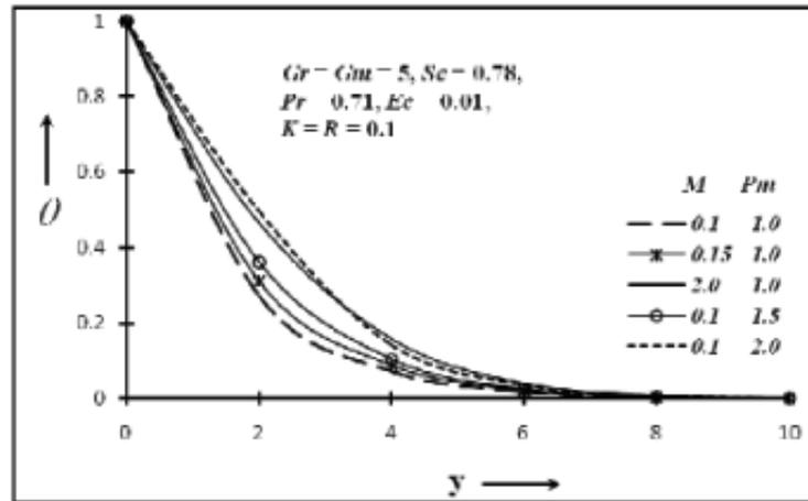
Fig. 3. Temperature field distribution with Hartmann and magnetic Prandtl number.
